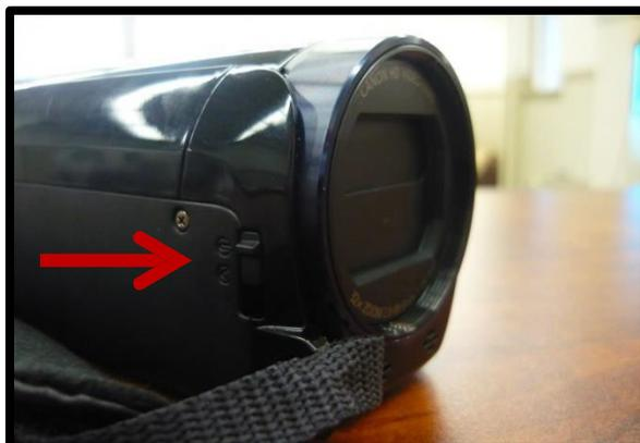
At the back of the camera, press the start/stop button to begin recording
