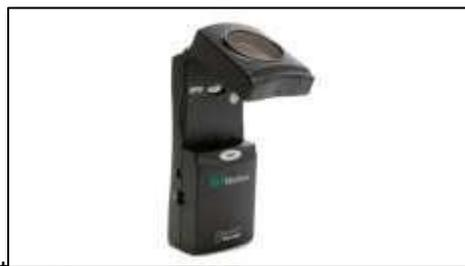
There are settings on the sensor that recognize slower motion and quicker motion, as represented by a person and a bus. For most experiments, you will use the slow (person) setting.
