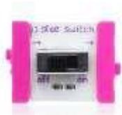
Pink bits are used as **input**, or action, bits—they *do* something. Switches, levers, dimmers, knobs, and many other input devices are available.
