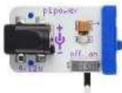
Blue bits are the **power** source bits. They usually include a battery connection, but there are also AC/DC adaptable bits and, recently, blue bits with USB ports have been created that can be run from the power in your computer.
