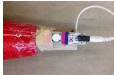
9. Tape the battery to the inside of the tube. This will prevent the battery from sliding out of the tube when you move around with the flashlight.
