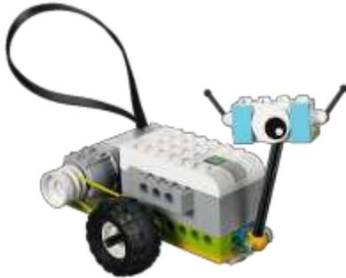
WeDos are lego sets that come with a power source and a motor that allows students to create lego constructions that move like robots. Once students create the robots, they can be paired with a device that is Bluetooth enabled which will allow students to control the robots. Students use simple block coding to program the robots as they desire.
