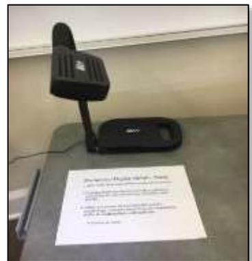
To connect the document camera to the desktop, take the small black USB 3.0 cable from the desktop station, and connect it to the USB 3.0 port on the document camera. The correct port is closest to the base of the neck.
