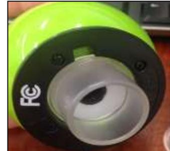
Place a slide or object on a flat surface near the Zoomy. Move the Zoomy over the slide or object and slowly lower the microscope until the image on the slide is magnified in the Xplovview software.
